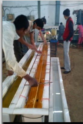
10 Ft. Long Bus bar Silver Plating Plant
