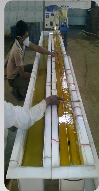
10 Ft. Long Bus bar Silver Plating Plant
